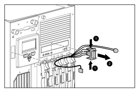
Figure 2-38. Removing the power switch
